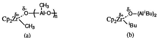
Figure 3. (a) Active species for the \text{Cp}_2\text{ZrCl}_2 -MAO catalyst system (b) Active species for the \text{Cp}_2\text{ZrCl}_2 -TIBDAO catalyst system
